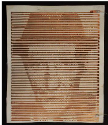
Figure 5. "Uncle Bill". A one-channel flat speaker on flexible magnetic sheeting.
