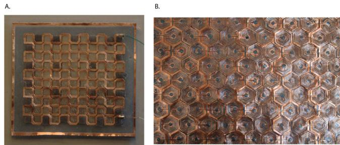
Figure 2. Two flat speakers designs using maximal tiling A. Square speaker. B. Hexagram speaker
