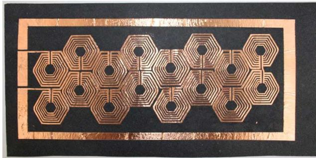
Figure 1. A flat speaker array of copper foil on paper
