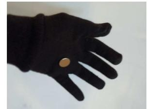
Figure 3. A Sound Glove with Magnet Attached
